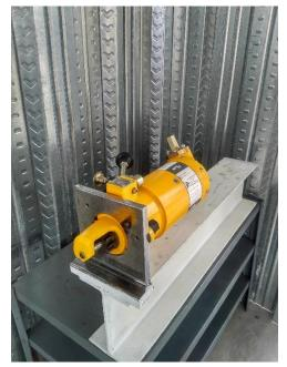
On some applications, the IPU spring starter is being tested while fitted to the storage bracket next to the engine.
