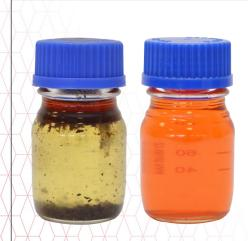
**Left:** a diesel sample we took from a customer before treatment. You can clearly see a layer of water with solid particulate build up at the bottom.
