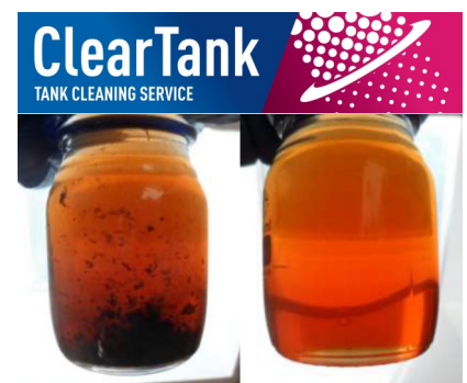
Fuel before (left) and after an IPU ClearTank service (right).
